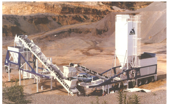
Mobile Batching Plant
