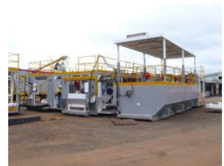
Ensign Energy services, QLD Mud pump skids Design, Drafting, Certification
