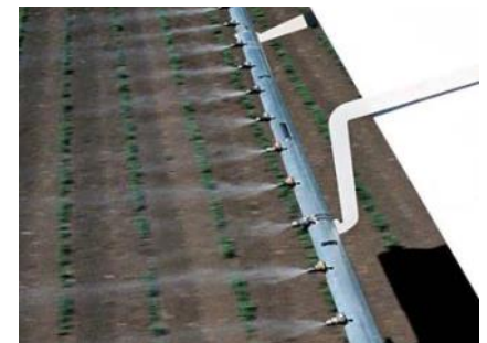
Jones Air St George QLD Rotating crop dusting boom Design, Drafting
